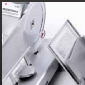
The carriage can be tilted for thorough cleaning
